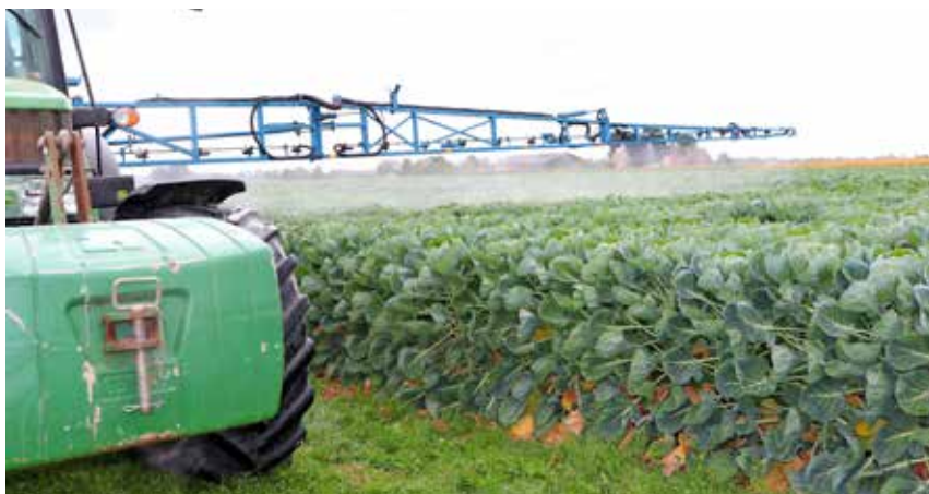
In spruitkool is de Wingsprayer ingezet met 1 of 3 doppen per 25 centimeter.
